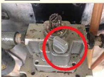
The cocks used before repairing the air leakage from the inner ring raceway grinding machine lubricator cock were made of resin and easy to break.
